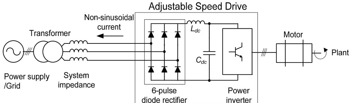
Over the years, many different harmonic mitigation solutions have been utilized. The simplest solutions consisted of passive filters, either series inductors or parallel capacitors, connected such that their impedance would block or sink the harmonic currents. Several other solutions emerged, such as pulse-multiplication, magnetic waveshaping, reconfiguration of the power system, and mixed non-linear loads.
