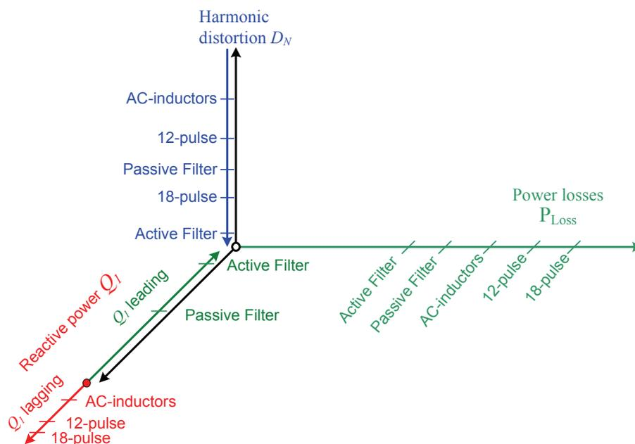
Regarding the power losses, the active filter has the lowest losses among the presented solutions. Being based on power electronics, the efficiency of active filters is significantly higher (estimated at
