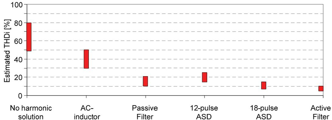
When comparing the performance between different harmonic solutions, the achieved  $THD_i$  is not the only decisive factor. As with any electrical equipment installed on the power system, all harmonic solutions have power losses and to some extent they generate reactive power (all passive solutions contain capacitors, inductors or transformers). The total apparent power has three dimensions: active, reactive and harmonic distortion power.
