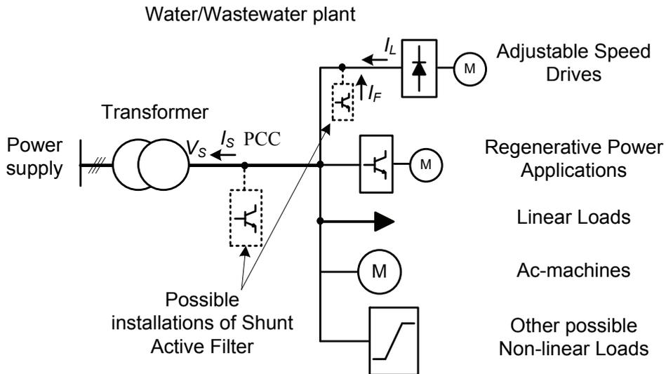
The efficiency is higher than that of a passive filter because the active filter provides harmonic current mitigation but does not load the network at the fundamental frequency. Unlike passive filters, there is no need for connecting multiple branches for mitigation of several harmonic orders at once. One single active filter is capable of mitigating up to a practical harmonic order of 30-50, meeting the actual harmonic standards and regulations.
