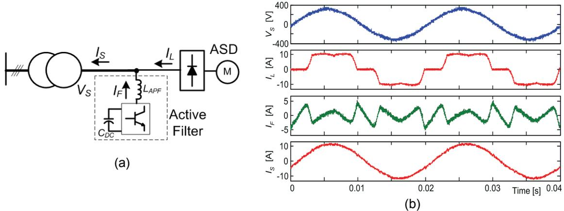
Possible connections of active filters on the power network are either close to the non-linear load (e.g., a high power VFD) or at the point of the common coupling (PCC) as a central harmonic solution serving multiple VFDs (Figure 3).
